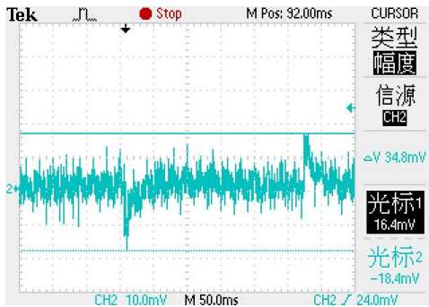
15. Load transient response (IL=10-350-10mA)
